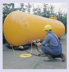
The compact power bags do their job even on round tanks: Placed alongside, they do the initial lifting for subsequent raising, recovery or transport.
