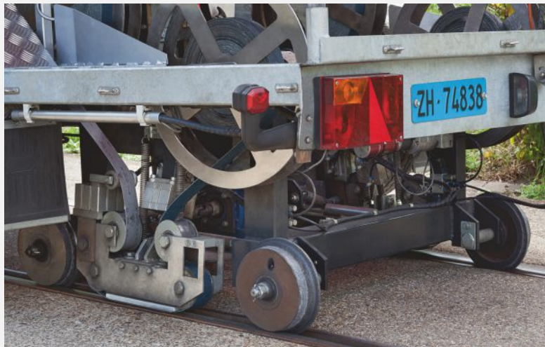
Thanks to the implemented belt-slip technology, the HGS module enables the removal of dirt such as ground-in leaves or grease from the rail head. An additional area of use is rolling contact fatigue, whereby a minimum amount is eroded from the surface of the rail.
