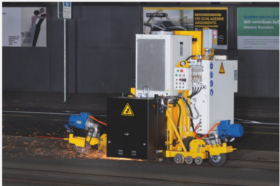
The AT 1003 rail grinding system consists of two grinding shafts and was constructed on an electrical basis. An external power source is required for use.
