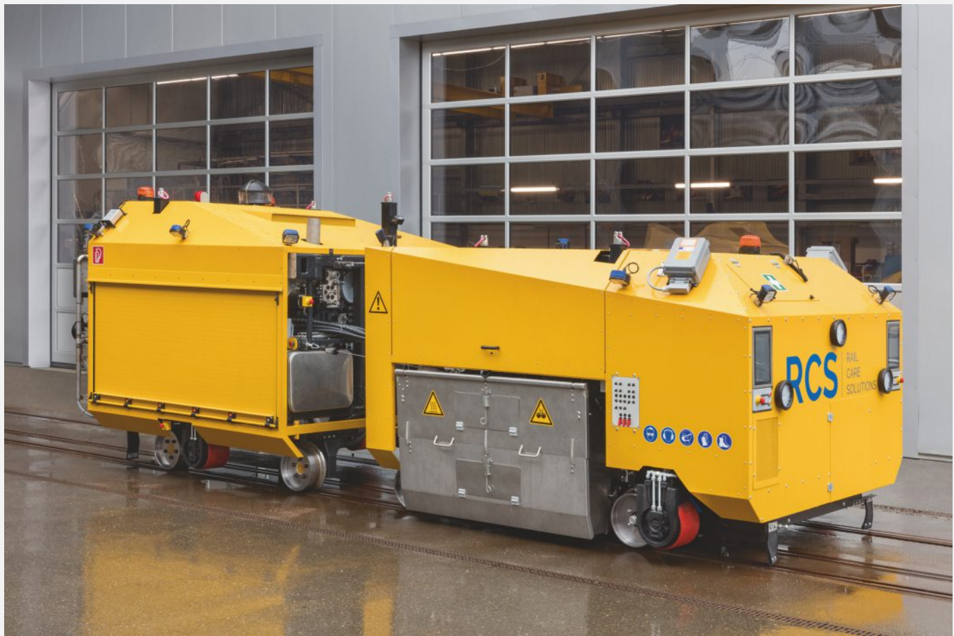
The autonomous AT 3389 rail grinding system was designed for grinding and reprofiling problem areas in grooved and Vignole rails. A thorough processing of switch equipment also makes an optimum servicing strategy possible. Due to its modular design, the system can be manufactured in different versions and with a varying number of grinding shafts.
