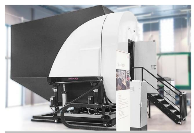
From 3 to 7 DOF, we provide any motion system to meet your needs. In the scope of this project, a 6DOF motion system is budgeted as an option (not contractual figure)
