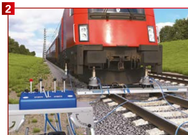
2 Two cylinders on the rerailing bridge bear the load
