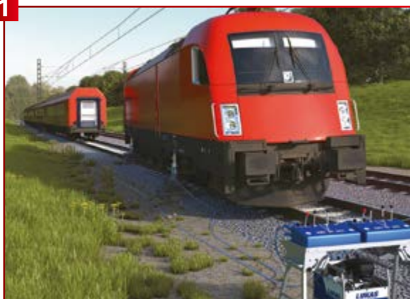
Lifting with 4 cylinders and horizontal alignment
