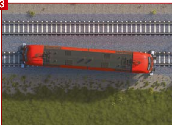
Possible to shift the rail vehicle simultaneously on two rerailing bridges
