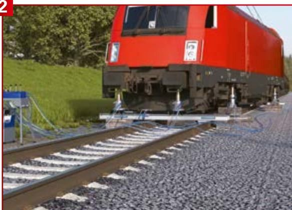
Four cylinders on two rerailing bridges bear the load
