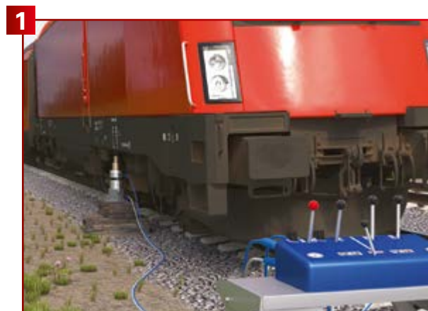
1 Lifting with 2 cylinders and horizontal alignment
