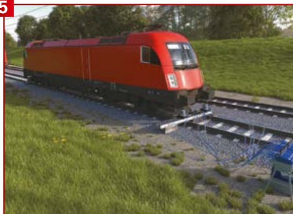
Lowering and rerailing the locomotive
